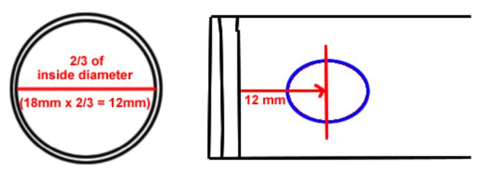
Note 1: we burn holes in bamboo rather than drilling because bamboo splits easily when drilled. When burning a hole, the iron tool should be red hot and generate large amounts of smoke. Try not to breath the smoke.
